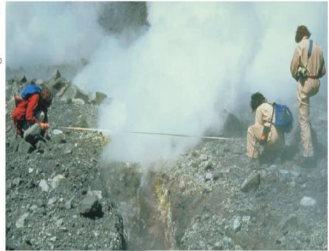
▶ SCIENTISTS USE A STEEL TAPE TO MEASURE THE CHANGES IN THE CRACKS ON THE CRATER FLOOR.
