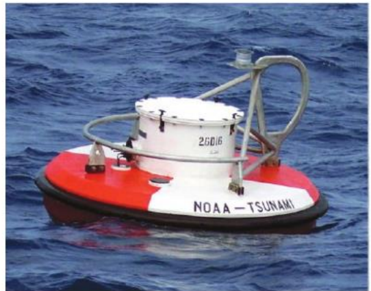
▶ BUOY THAT FORMS PART OF NOAA'S DART II SYSTEM
