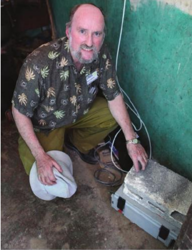
SCIENTIST DR. WALTER MOONEY INSTALLS A SEISMOGRAPH IN A VILLAGE BUILDING TO KEEP TRACK OF AFTERSHOCKS FROM THE 2010 EARTHQUAKE IN HAITI.
